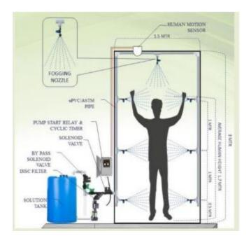
The tunnel creates a compulsory passage and is equipped with internal atomizing nozzles that saturate the environment with the biocide. It is connected to a control system that is capable of automatically mixing the sanitizing product. Access to the tunnel is regulated by motion detection.
